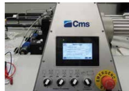
Software-based electronic control of cutting pressure
