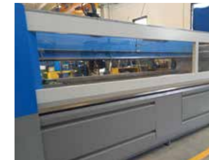
Front and rear hatch with pneumatic movement to better protect the cutting area and reduce the dispersion of water and abrasive material
