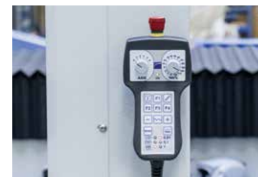
Remote pushbutton pad to control up to 6 axes that allow you to operate close to the cutting surface and set multi-origins (optional)
