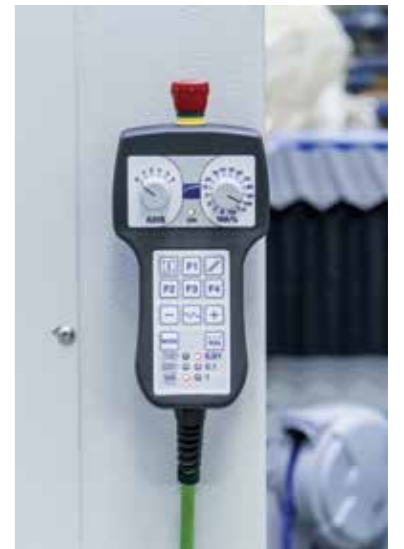
Remote pushbutton pad to control up to 6 axes that allow you to operate close to the cutting surface and set multi-origins
