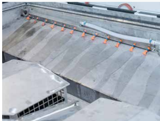
AUTOMATIC TANK CLEANING SYSTEM A set of nozzles positioned inside the tank that allow for processing debris to be conveyed to the external drainage filter
