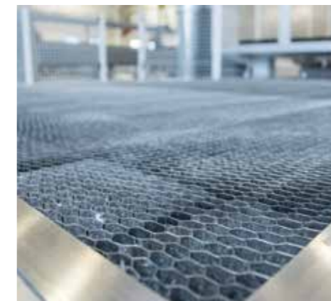
SUPPORT TABLE Alveolar grate in stainless steel for cutting plastic material.
