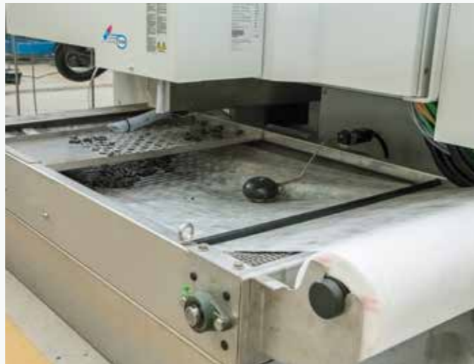
DRAINAGE WATER FILTERING SYSTEM An automatic system conveys the waste to the back of the machine where a paper filter with a collection tank cleans the waste water.
