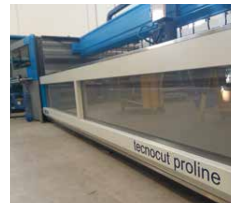
Front and rear safety doors with pneumatic movement to protect the cutting area and reduce the dispersion of water and abrasive material.
