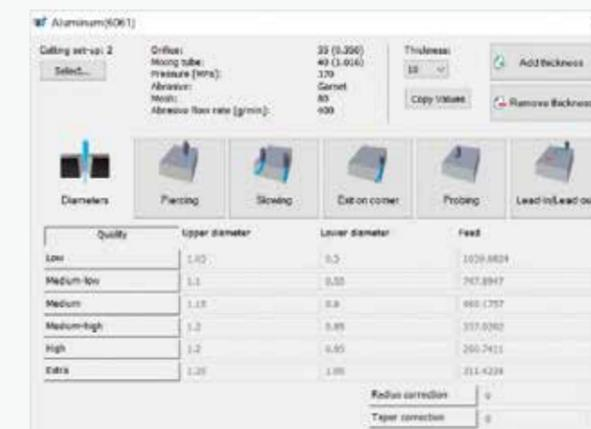
The JDE plug-in is included in the package to manage the cutting technologies archived in a complete materials database. The machine program is automatically generated on the basis of the selection of the cutting quality required out of 5 options (Q1, Q2, Q3, Q4 and Q5) that establish the speed advancement and acceleration settings in the internal/external corners. The ISO program can then be transferred to the machine using the local network or via USB drive.
