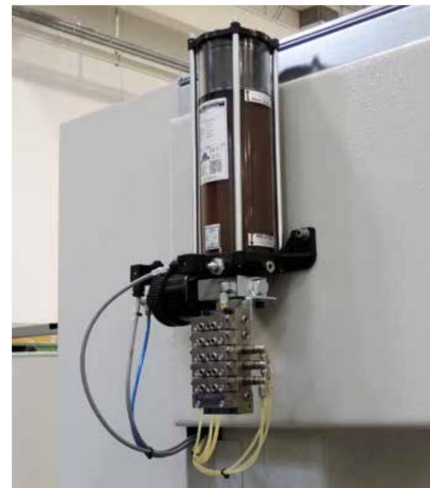
Automatic lubrication of all axes (std)
