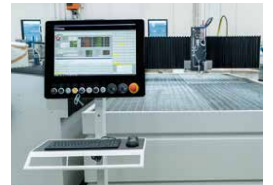
21,5" touch screen control panel on mobile trolley.
