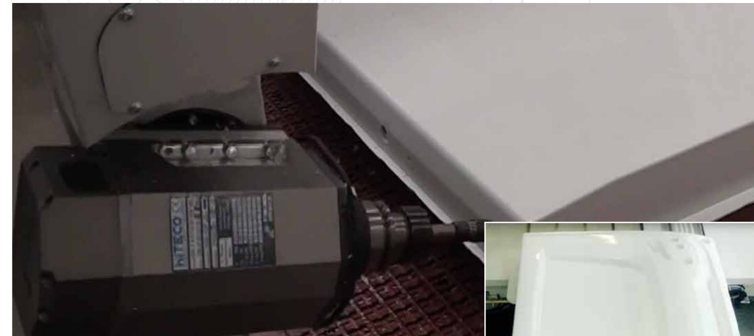
Trimming of thermoforming caravan components
