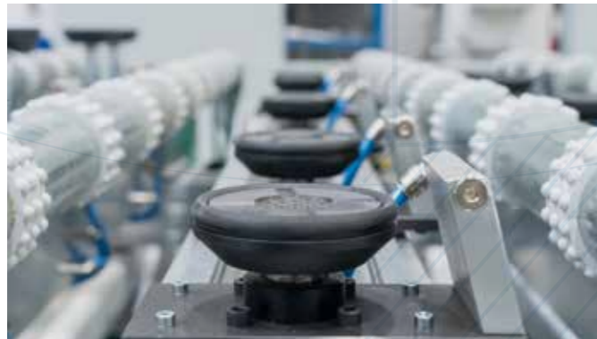
Suction cup with automatic cleaning system
