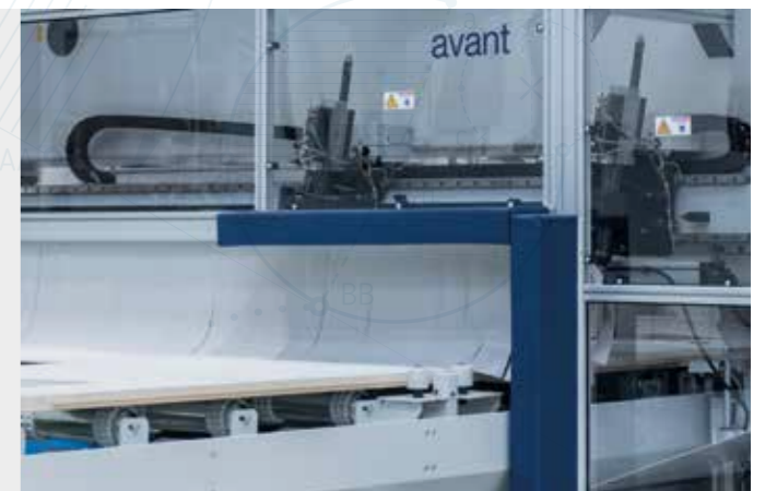
Rear pneumatic drills with adjustable center distance from CNC
