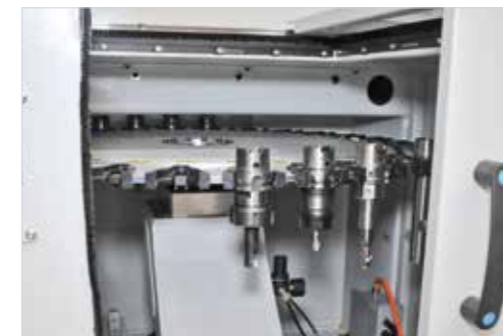
30 stations automatic rotary tool changer
