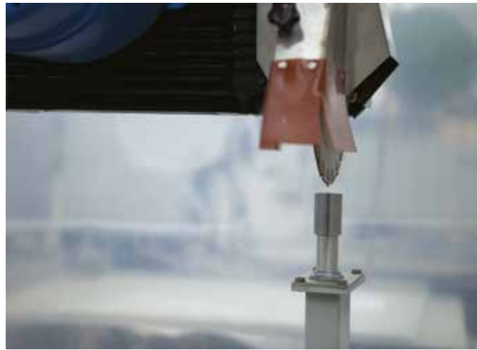
Presetter to measure the blade diameter and core drills/ milling length.
