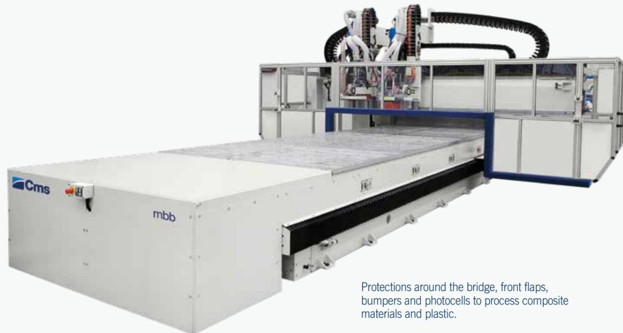
Protections around the bridge, front flaps, bumpers and photocells to process composite materials and plastic.
