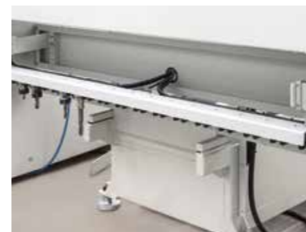
16 stations tool changer magazine
