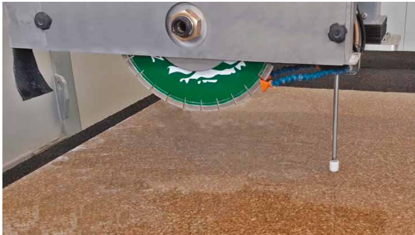
SLAB THICKNESS PROBE for the automatic measuring of the piece thickness
