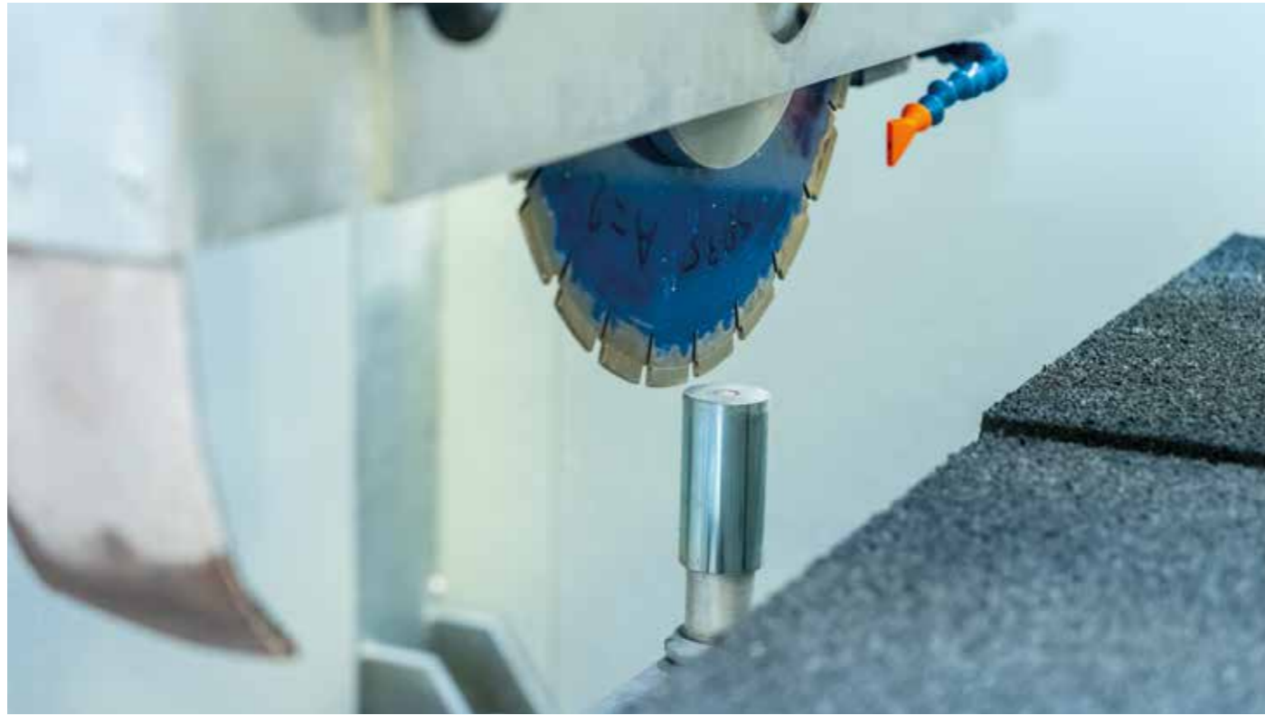
DISK PRESETTING to measure disk diameter and finger bits or core drills length
