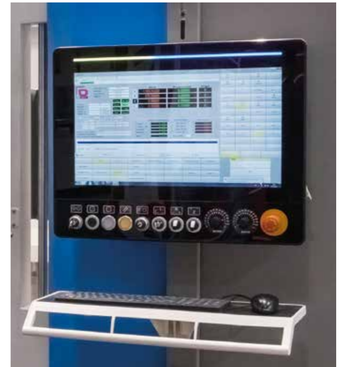
PC PANEL with touch screen controls and 21" screen
