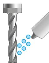
**Ionized air blower on the electrospindle**
