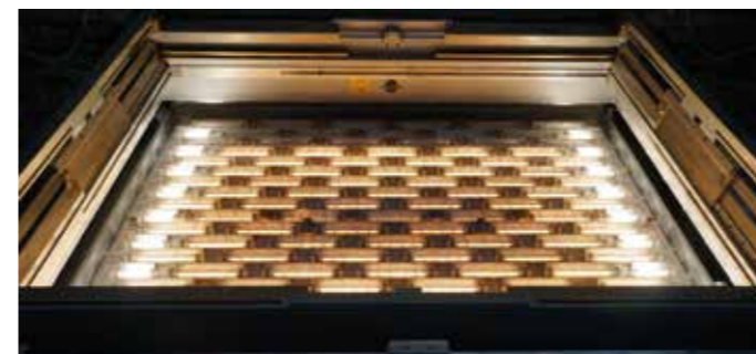
New heating system available with HTS Ceramic, quartz or halogen heaters: the power control is achieved in real time without continuity solutions for better adaptation to the material's thermal features. The current reading for each channel means faults can be identified quickly.
