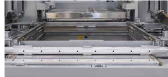
Automatic clamp frame: fully automatic adjustment system with telescopic crossbars. Guarantees cover to all the measurements without the need for manual set up, constantly guaranteeing maximum grip on the sheet.
