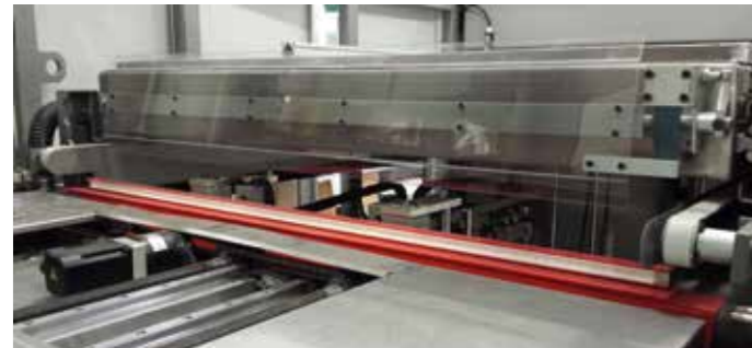
Sheet cleaning system with ionized air: eliminates electrostatic charges from each sheet and from the pallet installed in the loading zone. The utmost in terms of thermoforming quality and safety.
