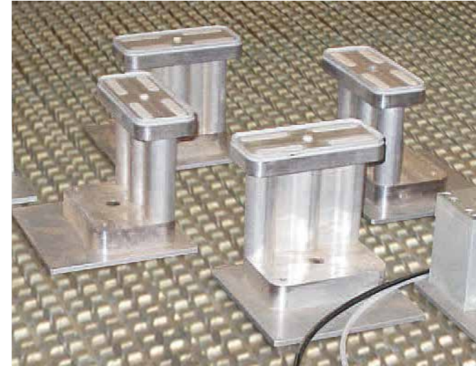
Suction cups and reference devices for maximum locking flexibility of the part.
