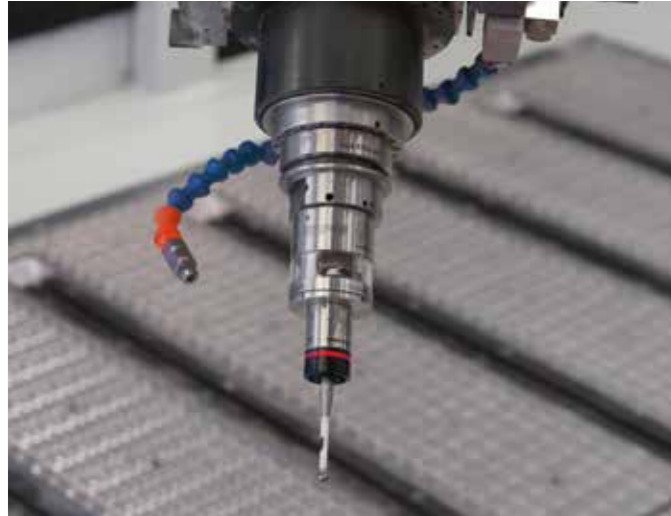
Probing device mounted on the toolholder with transmission of the signal via radio.
