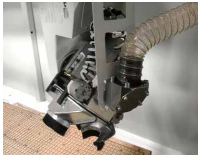
5-axis suction hood for concentrated suction on the cutting zone. Pneumatic opening for tool change and release.
