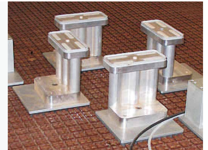
Suction and reference blocks for maximum flexibility in locking the piece
