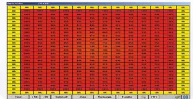
Variable heating power according to material temperature
