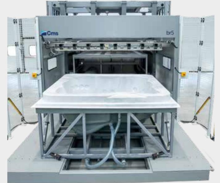
Heating system with double upper and lower panel with quartz elements
