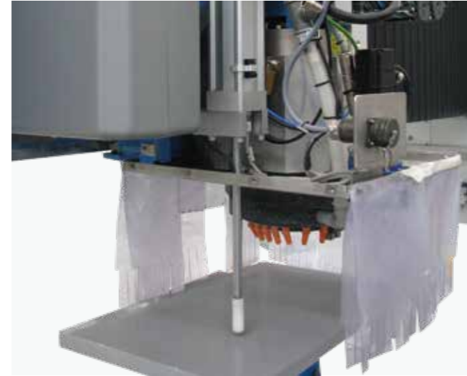
Thickness tester for capturing the actual thickness of the stone or ceramic slab to ensure the perfect execution of the piece.
