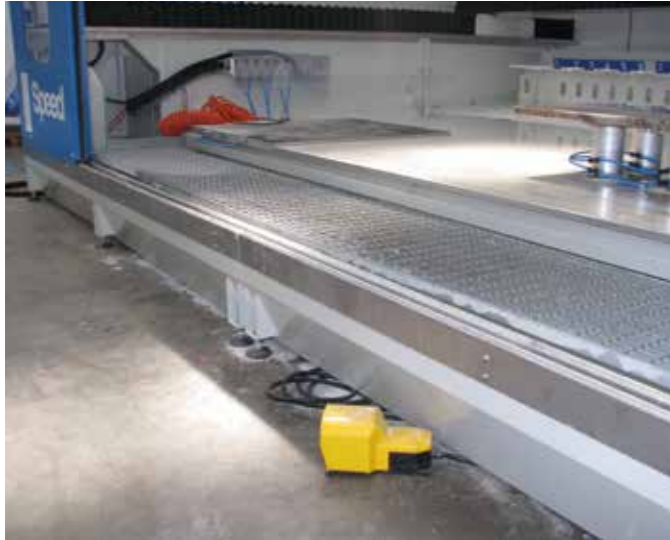
Front tank for processing water recirculation, complete with grated top to provide easy access for the operator.
