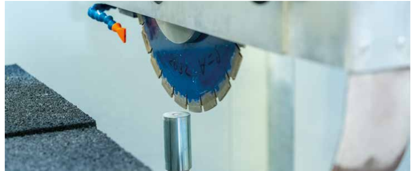
DISK PRESETTING to measure disk diameter and finger bits or core drills length
