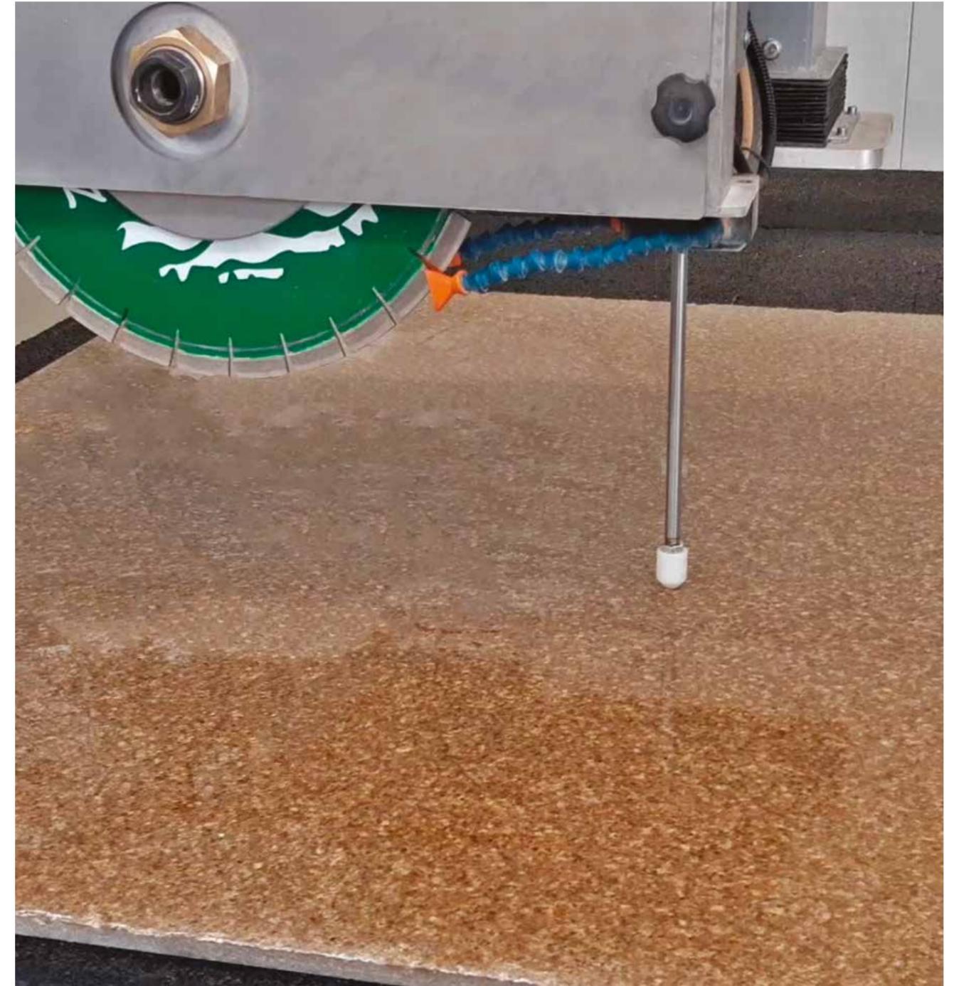
SLAB THICKNESS PROBE to automatically measure the thickness of the piece of stone or ceramic, this is essential in achieving perfect 45° cuts.
