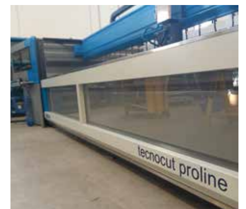
Front and rear hatch with pneumatic movement to better protect the cutting area and reduce the dispersion of water and abrasive material.
