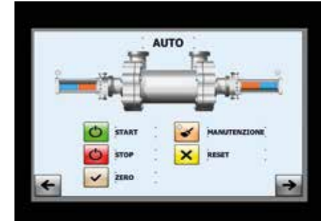
TOUCH CONTROL 17" for remote diagnostics, power check, cycle numbers and pressure electronic management (only on Tecnocut Greenjet Evo stand alone version)
