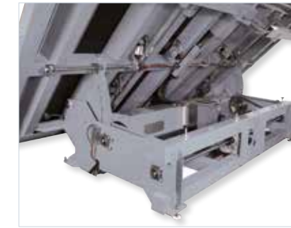
Mechanical tilting system. The automatic exit of loading feet is commanded during the work table tilting
