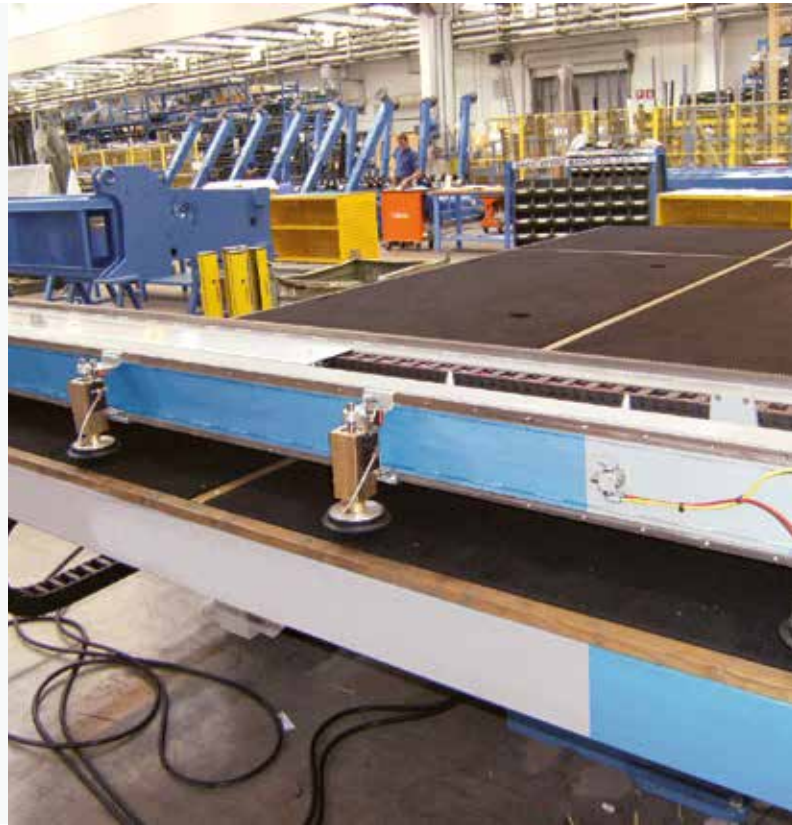
Suction cups for handling glass sheets (optional available only for Agil / Runner)
