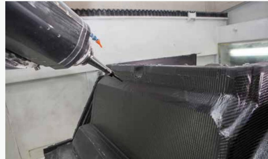
Structural component processing in carbon fiber.
