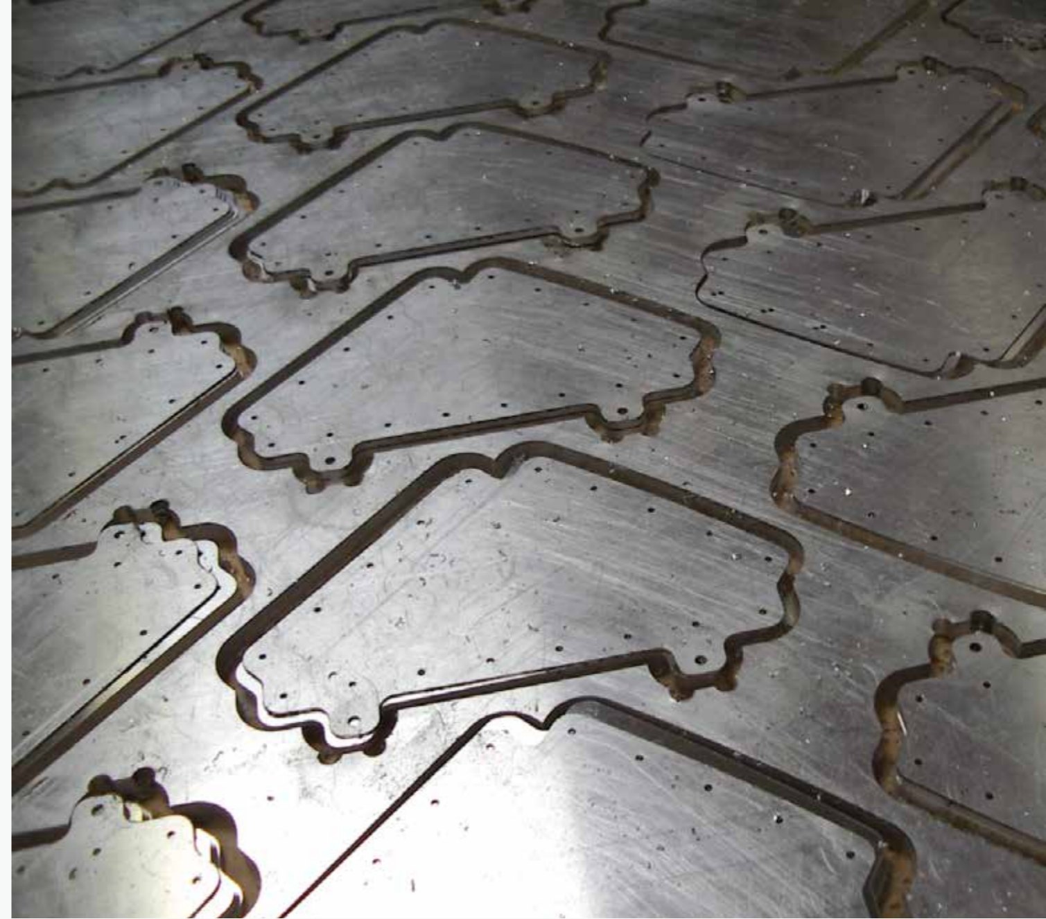
Stack machining of aluminum sheets
