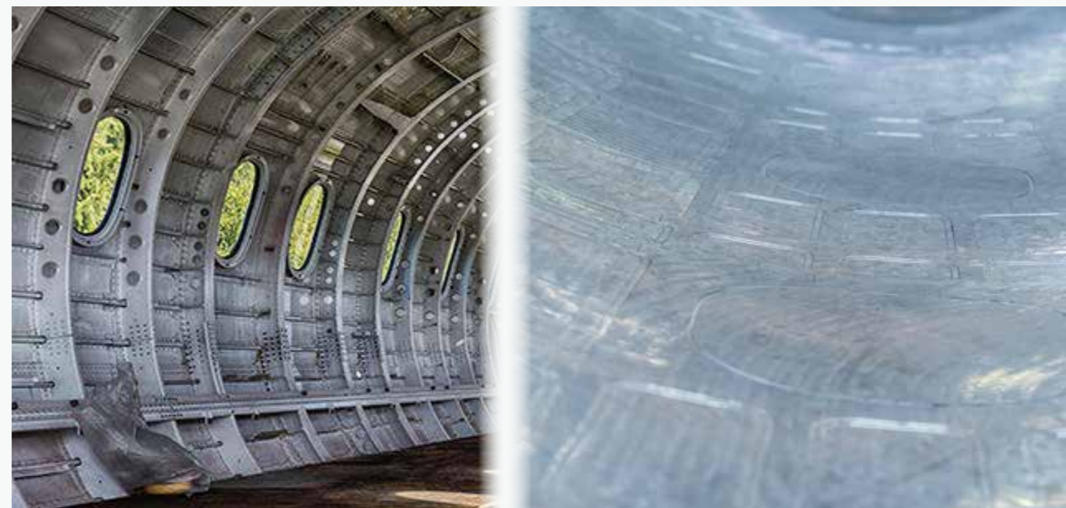
Surface milling of aluminum skins
