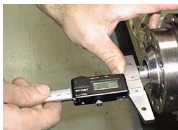
Figure 8 14. position of the expeller Figure 8 15. (A) expeller (B) reference position
