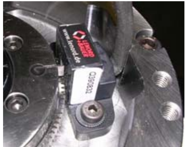
Lenord Bauer magnetic reader (sinusoidal wave)
