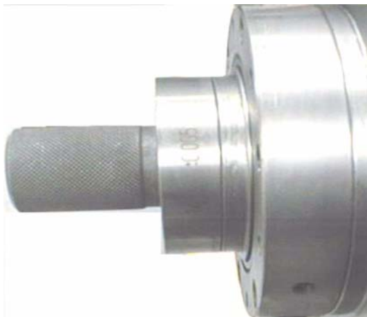
Figure 29: use of the gauge as a normal tool holder, with or without a thickness spacer interposed
