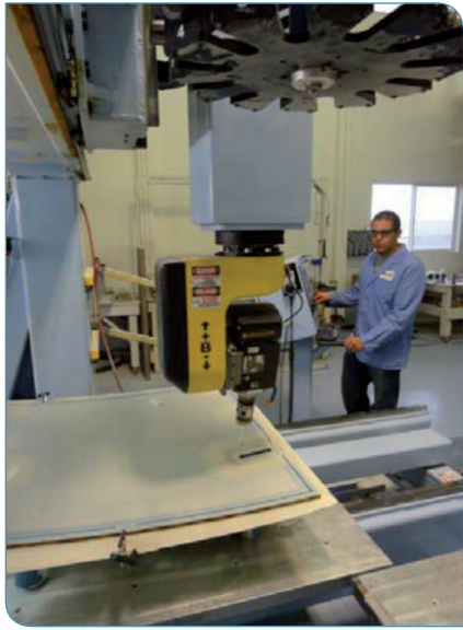
Fig. 3: DMS 5-axis CNC router machining a panel for the CH-47 Chinook helicopter at Unitech Composites
