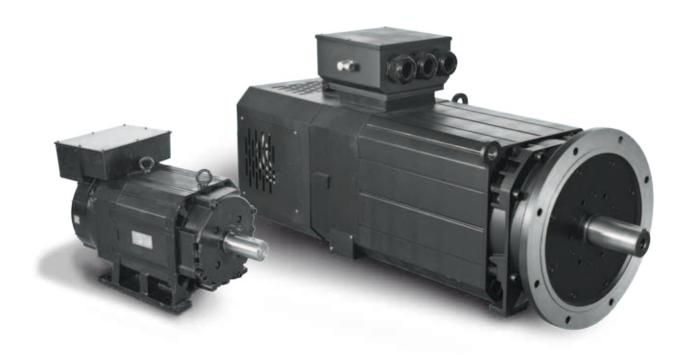
FM7 E01 - FM9 E01 motors have forced fan cooling and Delta (triangle) winding, with a rated power between 55 kW and 130 kW. They can reach speeds of up to 9,000 rpm.
