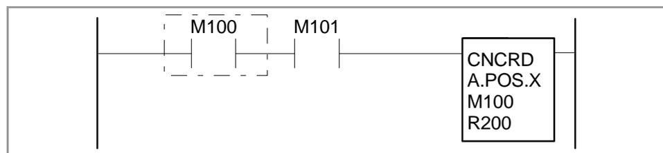
M100 AND M101 = CNCRD(A.POS.X, R100, M100)
