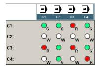
Channel 1 (CH1) is expecting synchronism marks from the rest of the channels. The marks of channels 2 and 4 are active. The mark of channel 3 is not active.
