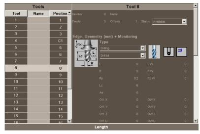
The left panel shows the list of available tools. For each tool, it indicates the position and the magazine where it is located, whether it is a ground tool or the tool is active in a channel.
