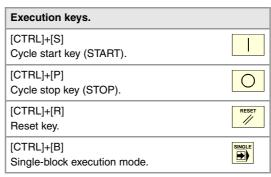
The shortcuts for the [START] [STOP] and [RESET] keys are only available when the CNC is installed as simulator on a PC.
