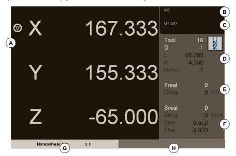
A Information related to the position of the axes. In the screen configuration supplied by Fagor, the data displayed will be different on each screen.
