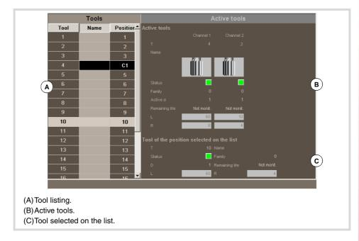
The left panel shows the list of the available tools and the right panel shows the data of the active tool in each channel.
