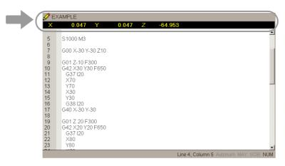
When TEACH-IN mode is active, it is possible to keep editing the coordinates of the axes directly from the keyboard or they may be assigned the current position of the machine axes. Both editing methods may be used indistinctly, even while defining a block. To define the coordinates of one or several axes using TEACH-IN:
