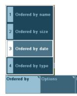
The softkey menu expands and shrinks with keys [F1] through [F7]. The softkey of the pop-up menu are selected with the [ENTER] key or from the numeric keypad using the number that comes with each softkey.
