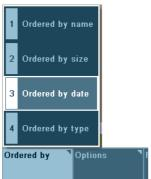
The softkey menu expands and shrinks with keys [F1] through [F7]. The softkey of the pop-up menu are selected with the [ENTER] key or from the numeric keypad using the number that comes with each softkey.
