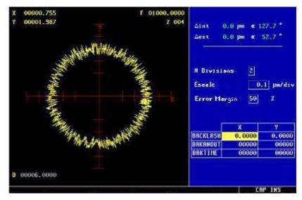
If the machine parameters are protected, it will request the access password because the bottom right of the screen shows some of them. When not knowing the password, those values cannot be changed, but it will be possible to access the screen and the circle geometry test.
