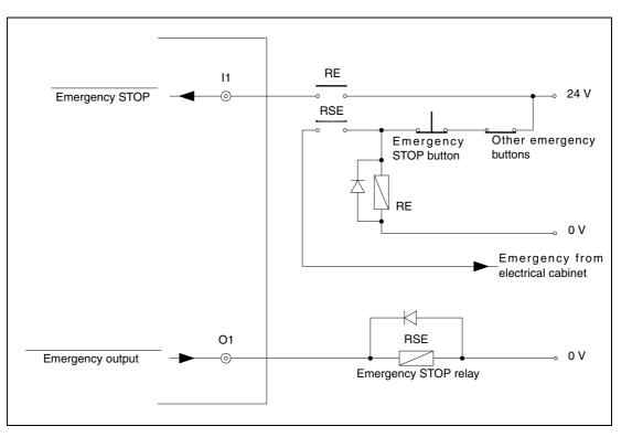
MACHINE AND POWER CONNECTION Connection of the emergency input and output
