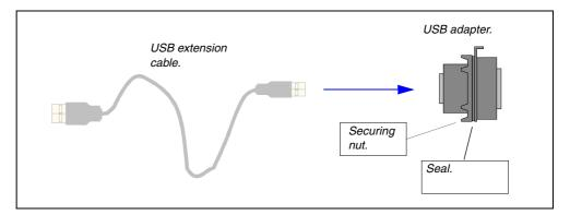
2. While the CNC is off, connect the extension cable to the USB connector of the CNC.
