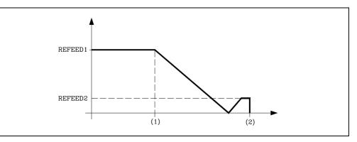
When the spindle does not have a machine reference (home) switch (s.m.p. DECINPUT (P31) = NO), the CNC will move the spindle at the feedrate set by s.m.p. REFEED2 (P35) until the first marker pulse from the current position is found, thus ending the home search.
