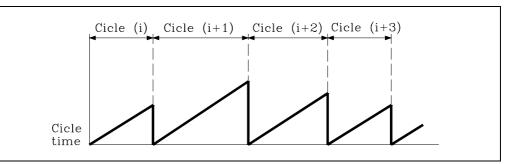
plc.m.p WDGPRG (P0) sets the maximum cycle execution time This is called WATCH-DOG time and if a cycle is executed which lasts longer than 1.5 times this time, or two cycles are executed, one after the other, taking longer than this time period, the CNC will display the WATCH-DOG error of the main module.
