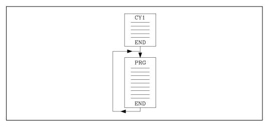
The periodic module will be executed every time the time indicated in the directing instruction "PE t" elapses. This count starts when the execution of the main module (the first time) begins.
