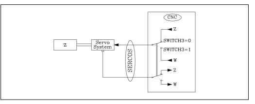
a.m.p. SWINBACK (P66) of the secondary axis must be set to "0".
