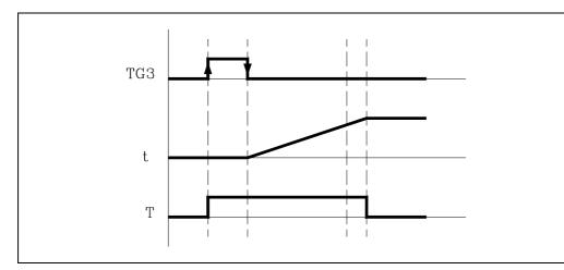
If the timer is initialized with values TEN=1 and TRS=0, the timer will be activated when a leading edge is produced at the TG3 input. At that moment, the timer status output will have a value of T=1.
