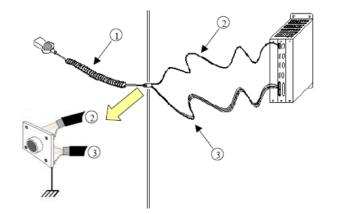
With the 8055 CNC, use a 7x1x0.14 PVC shielded cable for the feedback cable (2) of 5 V. The shield of both cables must be connected to the connector and to ground.
