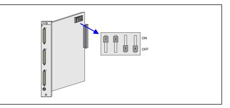
The logic address is set in binary code between 1 and 14. Logic address "0" and "15" are reserved. Logic addresses 0 and 15 are reserved.
