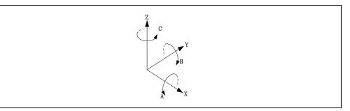
The rotary axes are called A, B or C depending on whether the rotation axis is X, Y or Z respectively. The turning direction of the axes may be changed with parameter "XFORM2".
