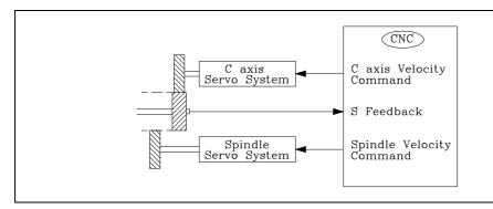
The feedback must be connected to the spindle (S) connector.
