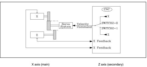
SWITCHAX for X = 0 SWINBACK for X axis = 0 Z axis (secondary) SWITCHAX for Z axis = 1 (X axis) SWINBACK for Z axis = 1
