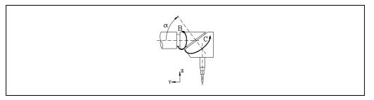
In an angular spindle, the main axis must be parallel to one of the axes X, Y, Z and the secondary axis will be at an angle with respect to it.
