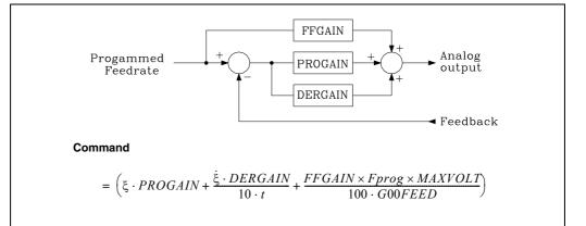
The feed-forward gain improves the position loop minimizing the following error, but it should only be used when working with acceleration/deceleration.
