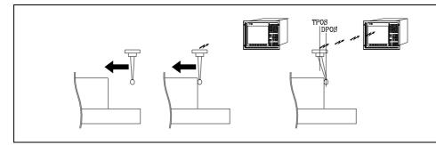
Although the probe keeps moving until the CNC receives the probing signal, the CNC takes into account the value assigned to general machine parameter PRODEL and provides the following information in the variables TPOS(X-C) and DPOS(X-C).
