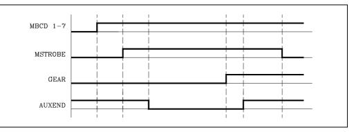
Once the general "AUXEND" input is activated, the CNC will require that this signal be kept active for a time period greater than the value given to the g.m.p. MINAENDW (P30).
