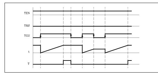
If, once the timing has finished, it is required to activate the timer again, another leading edge must be produced in the TG2 input.
