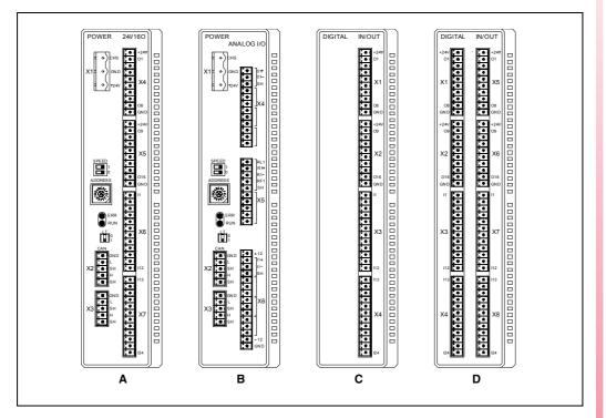
A. Power supply with 24 digital inputs and 16 digital outputs.
