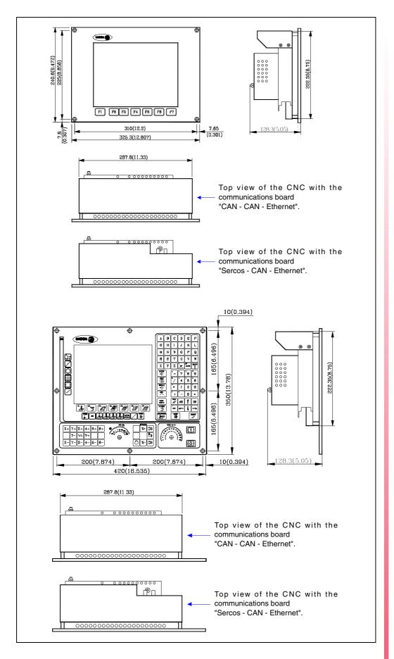
CNC 8055I CONFIGURATION CNC structure
