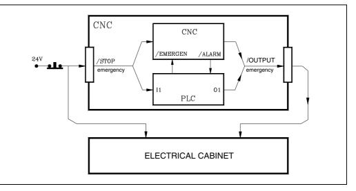
When the PLC sets the "/EMERGEN" input low (0V), the CNC stops the axes and the spindle and it displays the corresponding error message.
