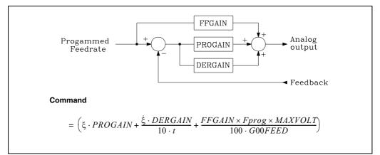
The feed-forward gain improves the position loop minimizing the following error, but it should only be used when working with acceleration/deceleration.
