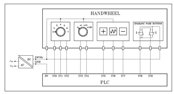
The example uses input I79, making it necessary to push both buttons in order to use the handwheel.
