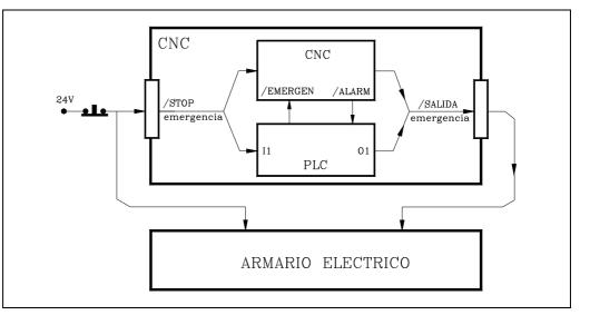
Likewise, while this signal is low, the CNC keeps the emergency output active (low).
