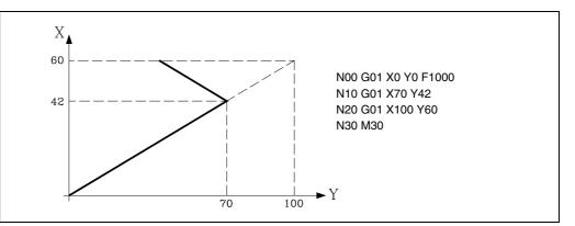
If, when executing the programmed movement in block N20 the signal corresponding to the X axis "MIRROR1" is active, the CNC will apply mirror image to the remaining movement in X.
