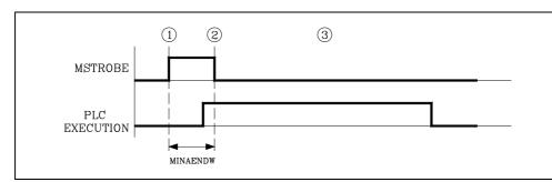
2. The CNC will keep the general logic output "MSTROBE" active during the time indicated by means of g.m.p. MINAENDW (P30).
