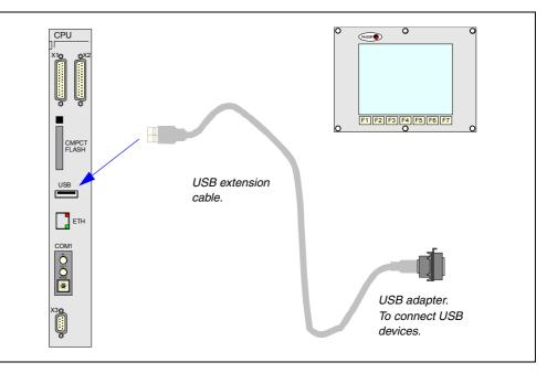
3. Once properly connected to the extension set, the USB devices may be connected through the adapter.
