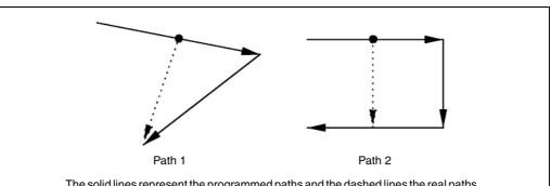
The solid lines represent the programmed paths and the dashed lines the real paths, after activating the BLOABORP mark.
