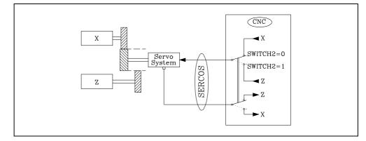
The CNC internally switches the feedback it receives via Sercos and it supplies it to either axis depending on the status of the SWITCH2 mark.
