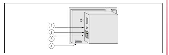
X1 SUB-D type 25-pin male connector to connect the video signals with the central unit.
