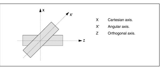
Programming in the Cartesian system (Z-X) requires activating an angular transformation of an inclined plane that converts the movements of the real (non-perpendicular) axes (Z-X'). This way, a movement programmed on the X axis is transformed into movements on the Z-X' axes; i.e. it then moves along the Z axis and the angular X' axis.
