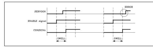
Also, if the SERVOON signal changes states during the movement of the axis, the CNC stops the axes feed and the spindle rotation displaying the corresponding error message.
