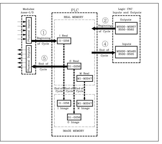
The following example shows how the PLC acts when working with real or image values.
