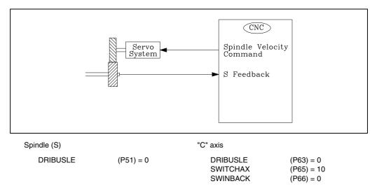
The feedback must be connected to the spindle (S) connector.
