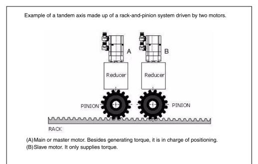
One of the many applications for the control of a tandem axis has to do with Gantry machines.
