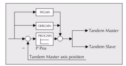
The values of PROGAIN, FFGAIN, DERGAIN of the master axis are applied to the slave axis; therefore, the gear ratios must necessarily be the same.
