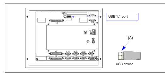
Use a USB extension cable to prevent undesired short-circuits with the metal housing (A) of the USB device at the CNC. The extension cable must not be longer than 3 m and it must be plugged in while the CNC is off.
