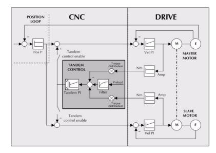
The block diagram has an area for the drive and another one for the CNC that comprises the position loop and the control of the tandem.
