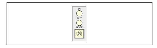
Each element integrated into the Sercos bus is identified with the 16-position rotary switch (0-15) "Address" (also known as Node\_Select). This rotary switch selects the address (node) occupied by each element integrated in the bus.
