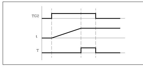
If the timer is initialized with values TEN=1 and TRS=0, the timer will be activated when a leading edge is produced at TG2 input. At that instant, the timing "t" begins from "0".
