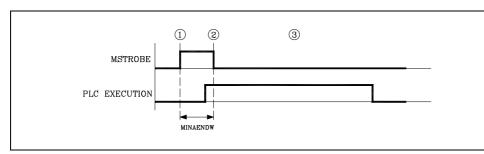
The CNC will keep the general logic output "MSTROBE" active during the time indicated by means of g.m.p. MINAENDW (P30).
