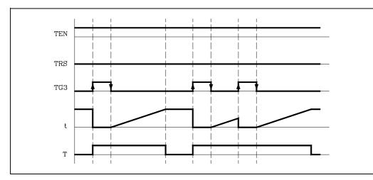
If, once the timing has finished, it is required to activate the timer again, another leading edge must be produced at the TG3 input.
