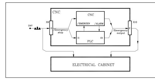
There are to ways to cause an emergency at the CNC, by activating the physical input /EMERGENCY STOP or the general logic input "/EMERGEN" from the PLC.
