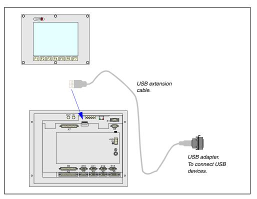
**3.** Once the extension set has been properly connected, it will be possible to connect and disconnect USB devices to the CNC while it is on.
