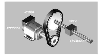
We have an axis with a maximum feedrate of 20 m/min, with a leadscrew pitch of 20 and a 3-to-1 gear ratio between the motor and the leadscrew. The motor encoder provides 2500 pulses per turn.
