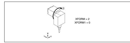
The swinging spindle head "XFORM=2" does not have a secondary or "dragged" axis but parameter "XFORM1" is defined like in the case of the  $45^{\circ}$  and spherical one.
