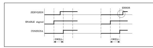
Also, if it changes to low during the rotation of the spindle, the CNC will stop the axes feed and the spindle rotation displaying the corresponding error message.
