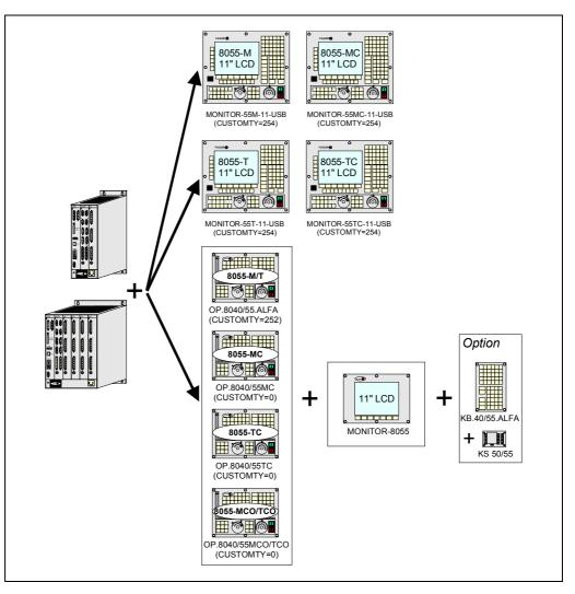
Use the video signal cable (up to 40 m) to connect the monitor with the central unit and the keyboard signal cable (up to 25 m) to connect the keyboard with the central unit.
