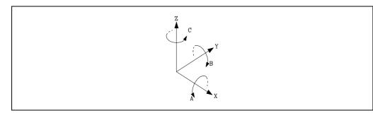
The rotary axes are called A, B or C depending on whether the rotation axis is X, Y or Z respectively. The turning direction of the axes may be changed with parameter "XFORM2".
