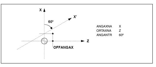
The axes defined in parameters "ANGAXNA" and "ORTAXNA" must exist and must be linear. These axes may have associated with them Gantry axes, coupled axes or axes synchronized by PLC.
