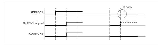
If the SERVOON signal is high, the CNC allows the movement of this axis by activating the ENABLE signal and providing the required velocity command output.
