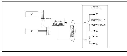
X axis (main) SWITCHAX for X = 0 SWINBACK for X axis = 0 Z axis (secondary) SWITCHAX for Z axis = 1 (X axis) SWINBACK for Z axis = 0
