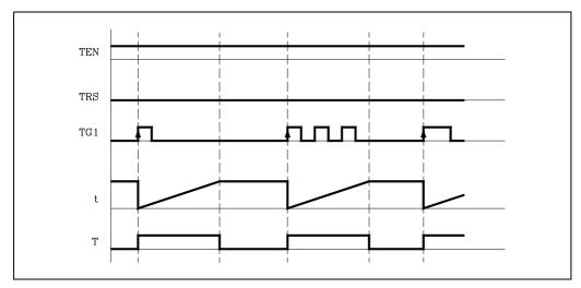
Once the time specified by the time constant has elapsed, timing will be considered as having finished. The timer status output (T) changes status (T=0) and the elapsed time will be maintained with the time value of the timer (T).
