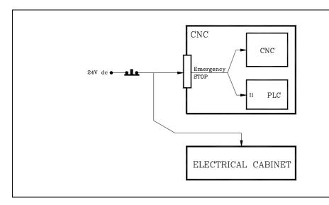
During the initializing process carried out by the CNC on power-up, the EMERGENCY OUTPUT of the CNC (pin 2 of connector X10) remains at low (at "0") in order to avoid a premature activation of the electrical cabinet.
