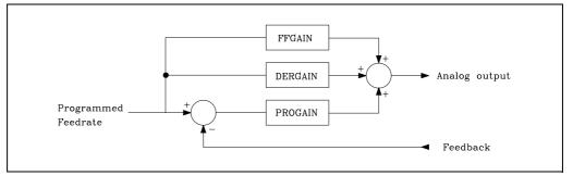
Best results are usually obtained when using it as AC-forward Gain, "ACFGAIN" (P46) = YES together with feed-forward gain.
