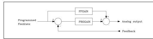
For example, if a.m.p. FFGAIN (P25) has been set to "80", the axis velocity command will be:
