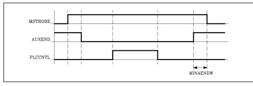
After analyzing the block and detecting the gear change the CNC indicates this to the PLC in one of the "MBCD1-7" registers (M41 to M44) and will activate the general logic output "MSTROBE" to tell the PLC that it must execute it.
