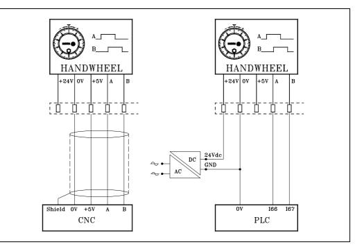
In the example on the left, the handwheel signals are taken to the feedback input (connector). Set the corresponding g.m.p. AXIS , for example: AXIS4(P3)=11.
