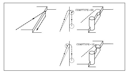
• At the end of the compensation, the tool should withdraw from the part without penetrating into it. The additional block must be executed in the upper plane and, consequently, together with the second block (COMPTYPE=10).
