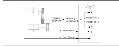
The two axes share the same feedback device. It must be connected to the feedback connector of the main axis.
