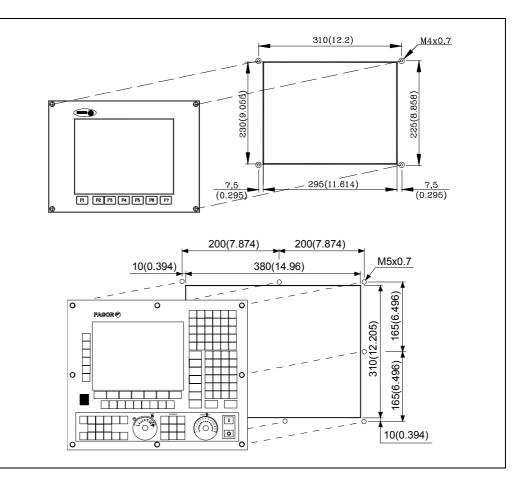
The minimum distance from each side of the monitor to its enclosure in order to guarantee the required ambient conditions is shown below:
