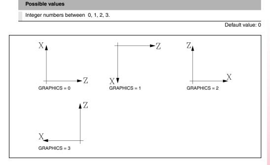
On M, MC, and MCO models, this parameter indicates the axis system being used for the graphic representation as well as the motion possibilities for the W axis added to those of the Z axis in the graphic representation (W additive).
