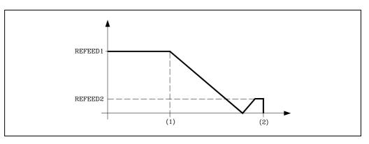
When the selected axis does not have a machine reference (home) switch (a.m.p. DECINPUT (P31) = NO), the CNC will move the spindle at the feedrate set by a.m.p. REFEED2 (P35) until the first marker pulse from the current position is found, thus ending the home search.
