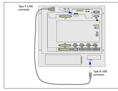
2. Once the extension cable is connected, it will be possible to USB connector of the front of the keyboard, while the CNC is on.
