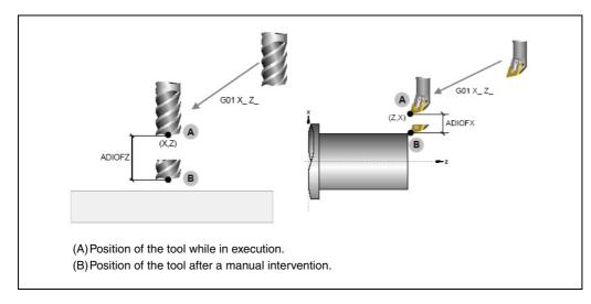
The intervention with an additive handwheel is only possible in execution mode, even while the program is interrupted. However, it is not allowed in the tool inspection mode.
