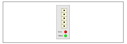
Each one of the elements integrated into the CAN bus is identified by the 16-position rotary switch (0-15) "Address" (also referred to as "Node\_Select"). This rotary switch selects the address (node) occupied by each element integrated in the bus.
