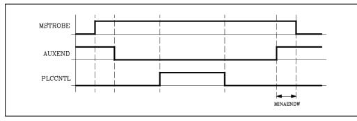
When the CNC detects a gear change, it sends out to the PLC the corresponding M code (M41 thru M44) via one of the logic outputs "MBCD1-7" (R550 thru R556).
