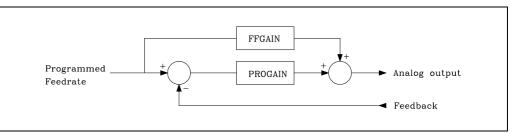
When it is due to variations of the programmed feedrate, "ACFGAIN" (P46) = YES, it is called ACforward gain" since it is due to acc./dec.
