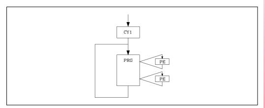
When defining the PLC program, both the processing of the main module (PRG) and the periodic modules (PE) must be taken into consideration.
