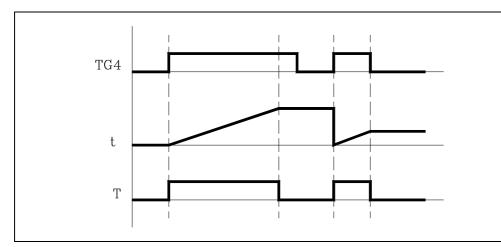
If the timer is initialized with values TEN=1 and TRS=0, the timer will be activated when a leading edge is produced at the TG4 input. At that moment, the timer status output (T) changes states (T=1) and the timing starts from "0".
