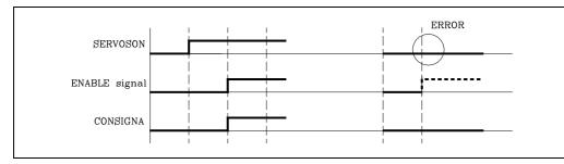
On the other hand, if the SERVOSON signal is low or if it changes to low during the rotation of the spindle, the CNC will stop the axes feed and the spindle rotation displaying the corresponding error message.
