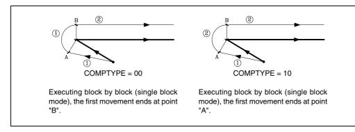
When the beginning or the end of the compensation takes place in a different plane (there is an intermediate vertical movement) and with angle greater than 270°, one should be analyze the CNC's behavior as shown next:
