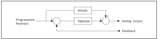
For example, if s.m.p. FFGAIN (P25) has been set to "80", the spindle velocity command will be:
