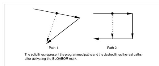
If a block is aborted and then the RETRACE function is activated, the retraced path (backwards) will not be the same as the one traveled forward. The two paths will not coincide either when aborting a block while the RETRACE function is active.
