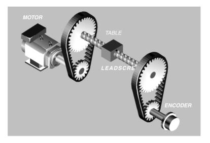
We have an axis with a maximum feedrate of 20 m/min, with a leadscrew pitch of 20 and a 3-to-1 gear ratio between the motor and the leadscrew. The encoder is an HOP model (Vpp) and provides 18,000 pulses per turn and a 2-to-3 gear ratio.
